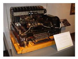
Figure: A Siemens and Halske T52D cipher machine on display at the Imperial War Museum, London. Source: https://commons.wikimedia.org/wiki/File:T52-iwm.jpg
